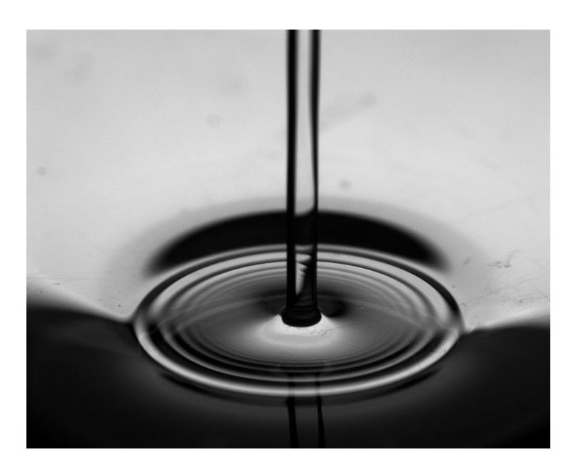
Hydraulic jump is an old free surface flows problem, where arise a sudden transition from high speed, supercritical flow to a subcritical one, with a sudden jump of the fluid depth.
