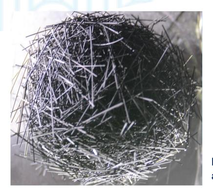
Nylon flexible fibers of aspect ratio 25-100.
