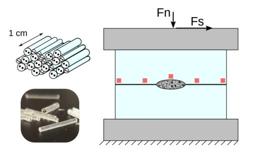
**Experimental setup :** 2D solid-solid friction with a perturbative granular patch
