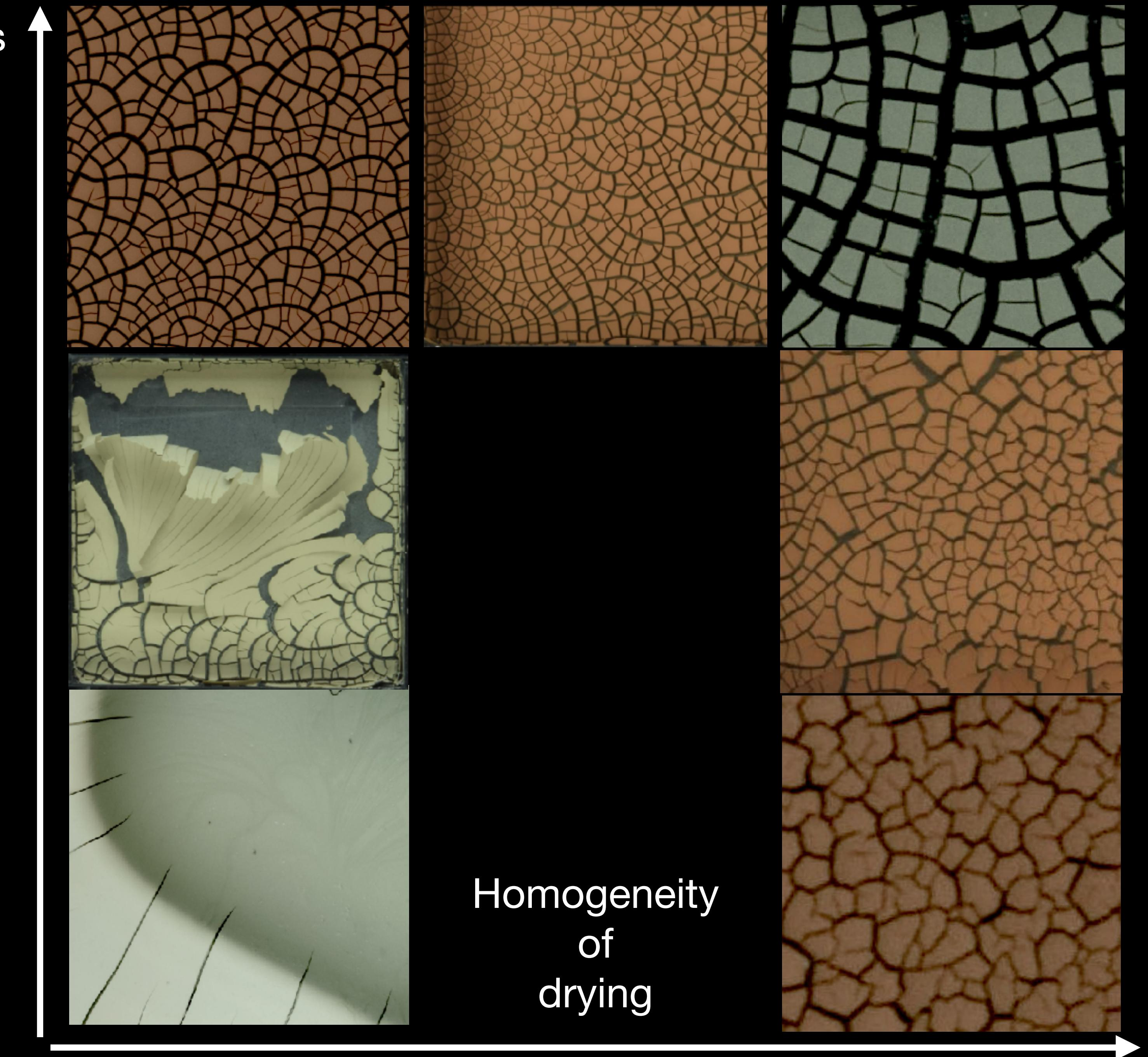
Model for cracks propagation
