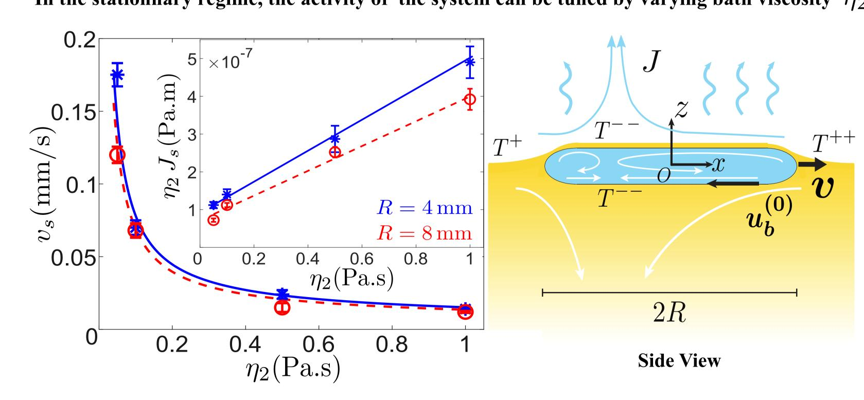
Evaporation is governed by two transport processes of vapour in air, diffusion and convection.
