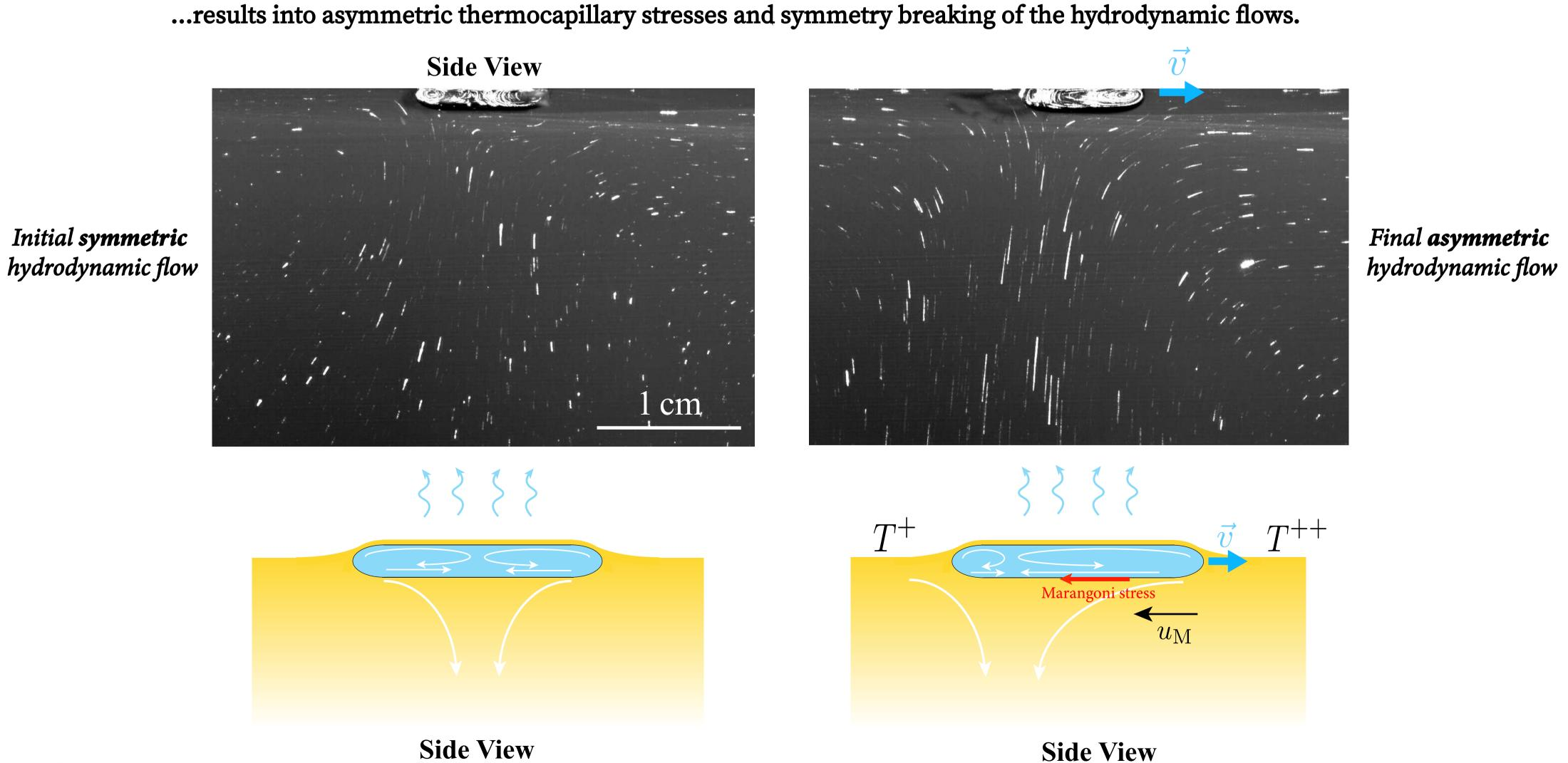
A propulsive force emerges as a result of the viscous stress response of the liquid bath
