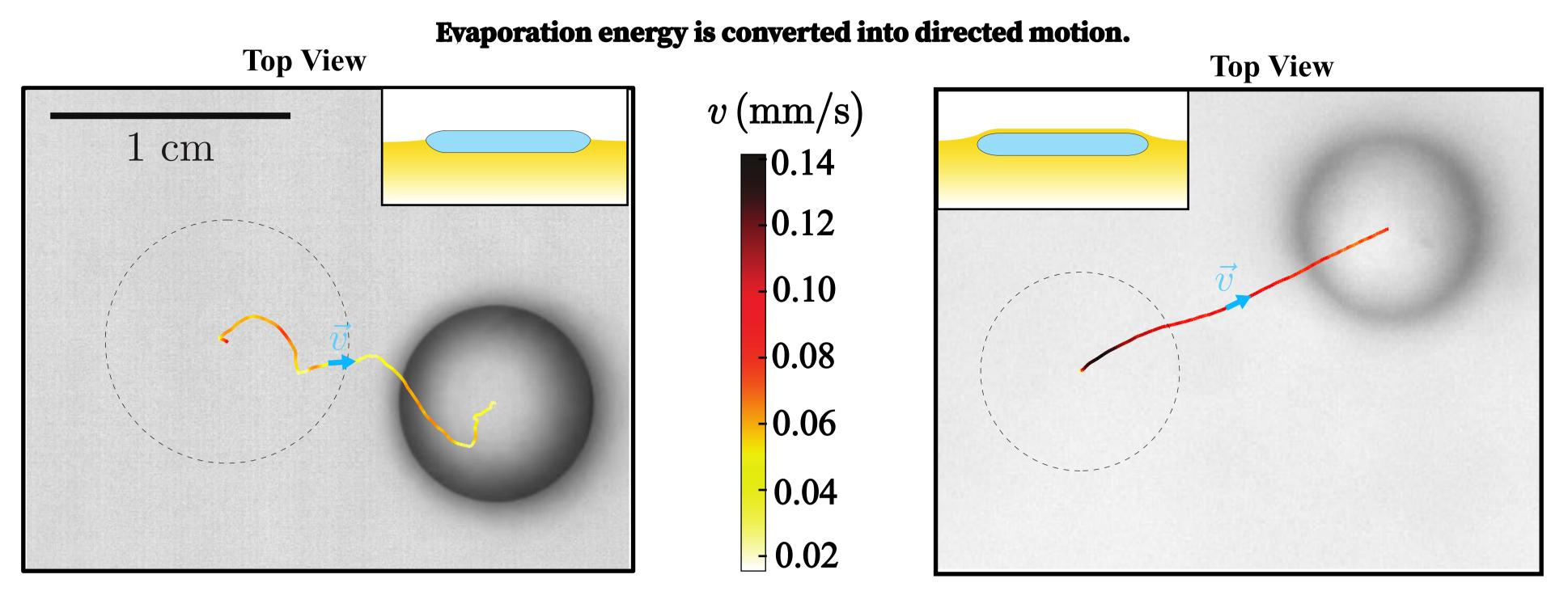
The presence of a thin film of bath liquid coating the drop is associated to straighter trajectories.
