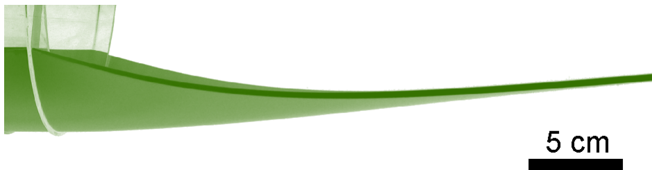
Figure 1. Side view a rectangular elastic strip (length 30 cm, width 20 cm, thickness 3 mm) pressed against a circular cylinder of radius 10 cm.
