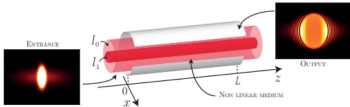
Stationary propagation of the complex amplitude of the electric field :
