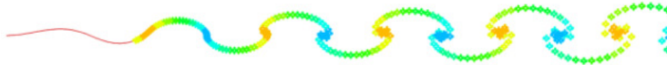
Figure 1. Self-propelled swimmer using vortex panel based FSI approach with wake particles colored by vorticity, orange positive, blue negative.
