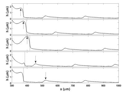
Periodic time evolution of the meniscus edge Vsub = 30  $\mu$ m/s,  $f_o$ =0.01,  $\tau$  = 8.69s. The black arrow indicates the bump top. The vertical dotted line is the position of the drying front.
