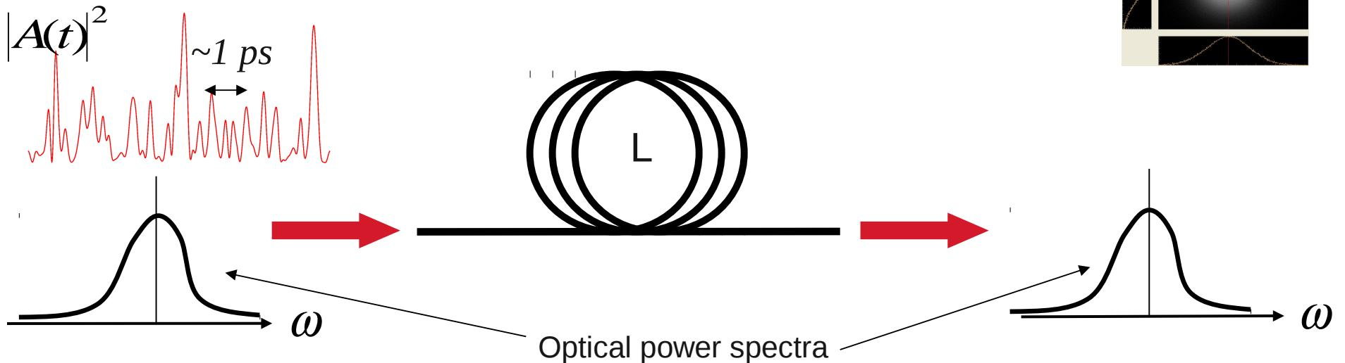
$$i \partial_z \psi(z, t) = -\frac{\beta_2}{2} \partial_t^2 \psi(z, t) + \gamma |\psi(z, t)|^2 \psi(z, t)$$
